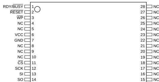
TSOP Top View – Type 1
